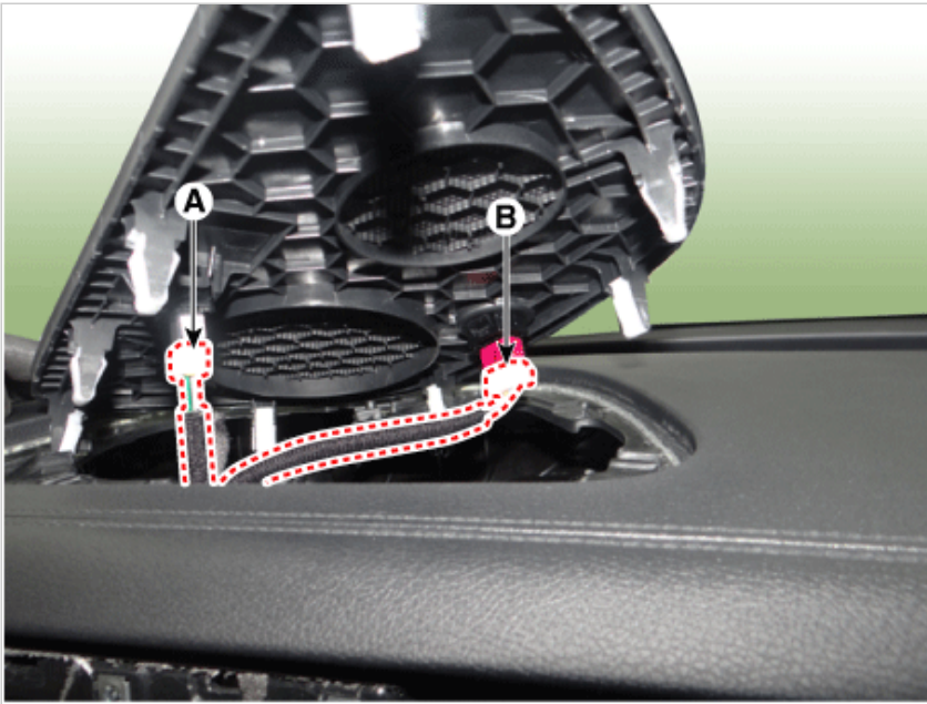
4. Remove the crash pad center speaker (A) after loosening the mounting screws.
